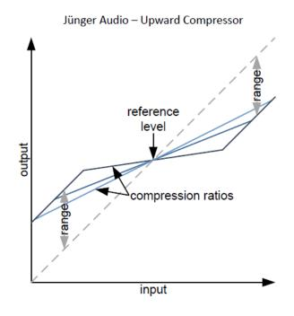
Microdynamic structures are maintained over the entire range of the input signal level. Even after compression the transients remain preserved. Although producing an output signal that is condensed in technical terms, the Jünger compression algorithm leaves a transparent, seemingly uncompressed sound impression.
