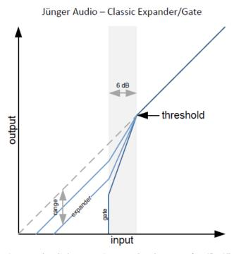
In the older design, downward expansion is increased over a level range of 6 dB. All signals below this range are attenuated by the range value.
