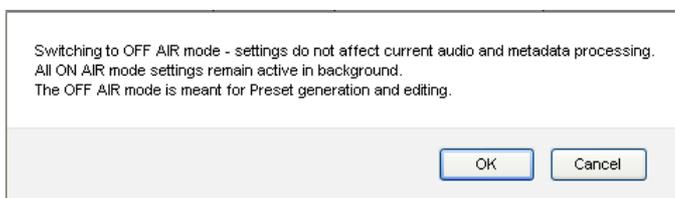
If you hover with the mouse over that switch in **OFF AIR** mode the hint: **"Processing is active, but settings are offline"** will be displayed.
