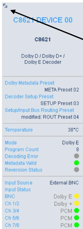
If you are controlling a specific module you will see a status frame on the left hand side that also appears if you hover with the mouse over the graphical boxes in the GUIs **OVERVIEW** display. If the GUI size does not fit your screen well you may reduce the size of the status display by clicking on the little arrows in the upper left hand corner to get a smaller view.
