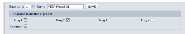
Tick the check box(es) for which program this preset shall be saved and press **<SAVE>**.
