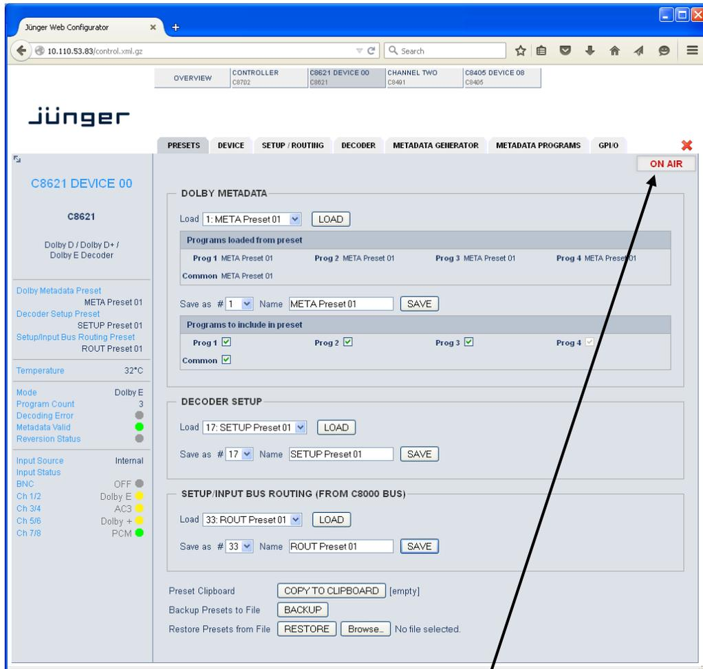
**Important Note!** The module may be controlled in **ON AIR** mode ● I.e. all settings have immediate effect. While in **OFF AIR** mode you may prepare presets without affecting the current operation. In this case online functions like preset clip board are not available.
