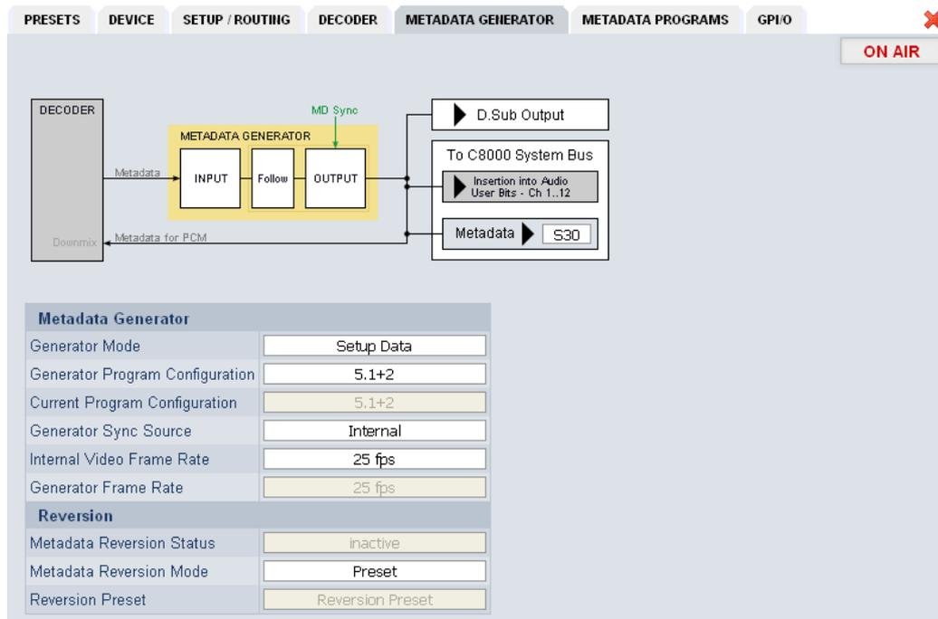
The **C8621** provides an extra metadata generator that can be used transparently (decoded metadata appear at the outputs) or controlled via the setup data. In the latter case the output metadata may be derived selectively from the decoder.
