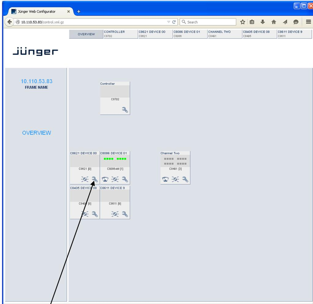
Clicking on the ● **spanner tool** within the module graphics of the **C8621** will open the pages of that module.
